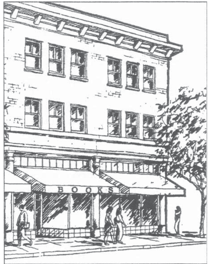
Figure 29: Awnings should be designed as integral parts of the façade; they should complement the architectural style of the building and fit within enframed storefronts.
