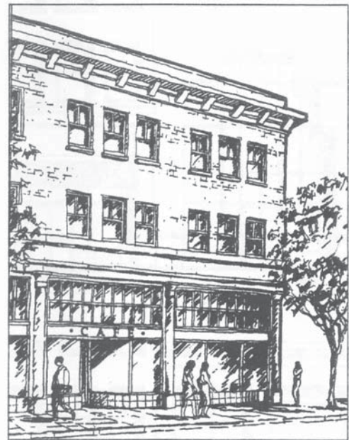
Figure 10: This façade composition, typical of Landmark and Significant buildings, shows how the ground floor is distinguished from upper floors, and how a consistent rhythm of storefront bays is maintained along sidewalk.
